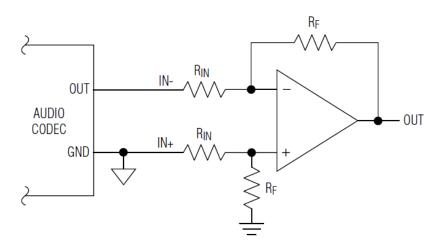
Fig. 3 Single-ended Input Configuration
