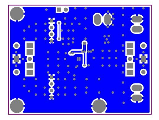
Fig.5 Bottom View of HT97220 Demo Board PCB Layout
