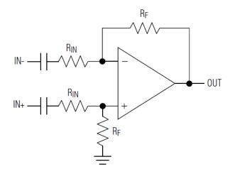
Fig. 2 Differential Input Configuration
